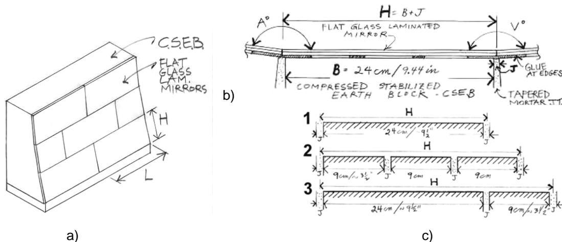
**Fig. 3-** Flat glass laminated mirror CSEB test wall: a) small test wall; b) section of flat glass reflector glued to masonry; c) CSEB masonry course sizes with selected block and mortar joint sizes.
