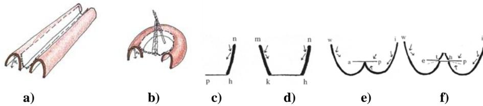
**Fig. 1- BUILDING SIZE FIXED REFLECTOR CPC TROUGHS and BOWLS for FOOD PROCESSING FACILITIES:** a) CPC trough; b) solar bowl; c) one sided CPC; d) CPC; e) involute; f) split involute.
