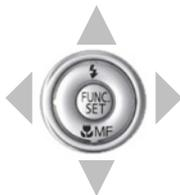
Use UP / DOWN directional buttons to highlight, FUNC.SET button to select a folder, RIGHT button to select a file, LEFT button for pop up menu for Cut, Copy, Delete, Select Inverse, RAW sum, RAW average, Purge RAW, Sub from marked, DNG -> CHDK RAW.
