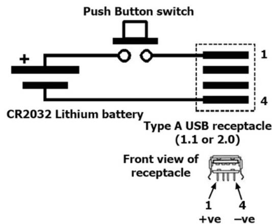
If you are cutting up a commercially-made USB extension cable, then wires 1 and 4 are red and black, respectively, according to the USB standard. It seems that even cheaply made USB cables follow this standard. Recent cameras have a combined USB and AV connector, a "splitter" type cable & connector is required.
