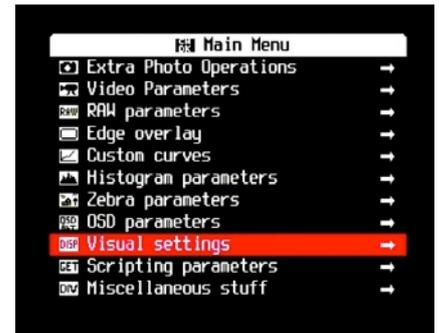
Like Canon's menus, pressing the FUNC.SET button will select the highlighted menu option. Pressing the DISP. button will move back one menu level. Pressing the MENU button will exit the current operation.
