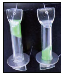
WAPI before and after reaching 65°C
